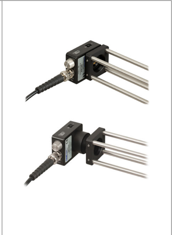
These two pictures show a DET series photodetector in a horizontal configuration. The top picture shows the detector directly coupled to a CP02 cage plate. The bottom picture shows a DET series photodetector attached to a CP02 cage plate using an SM1T2 adapter in addition to the SM1T1 that comes with the PDA series detector.
