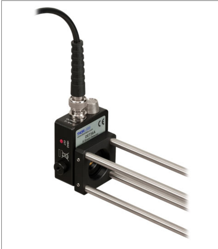
This picture shows a DET series photodetector attached to a CP02 cage plate after removing the SM1T1. The retaining ring from the SM1T1 was used to make the orientation of the detector square with the cage plate.
