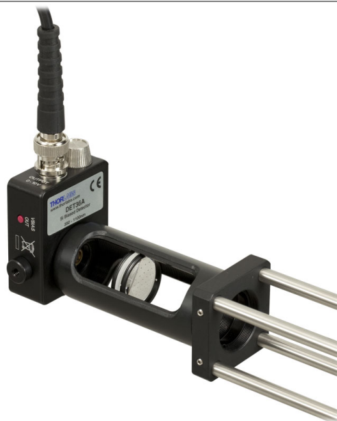
DET series photodetector mounted onto an SM1L30C Ø1" Slotted Lens Tube, which is housing a focusing optic. The lens tube is attached to a 30 mm cage system via a CP02 SM1-Threaded 30 mm Cage Plate. This arrangement allows easy access for optic adjustment and signal alignment.
