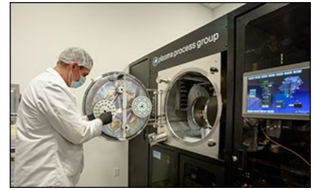
Ion Beam Sputtering (IBS) Chamber for Ultrafast Optics
